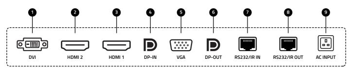
① DVI - ② HDMI2 - ③ HDMI1 - ④ DP-IN - ⑤ VGA - ⑥ DP-OUT - ⑦ RS232(RJ45)/IR IN - ⑧ RS232(RJ45)/IR OUT - ⑨ AC INPUT
